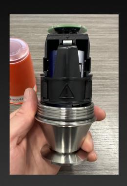
1 Remove the top cover by carefully twisting off
