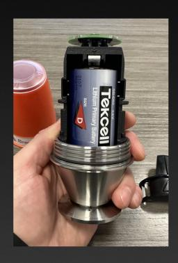
2 Remove the battery retaining clip
