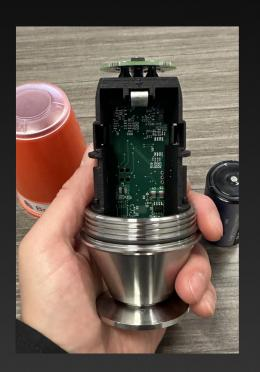
3 Remove the battery by pulling forward and down from the top
