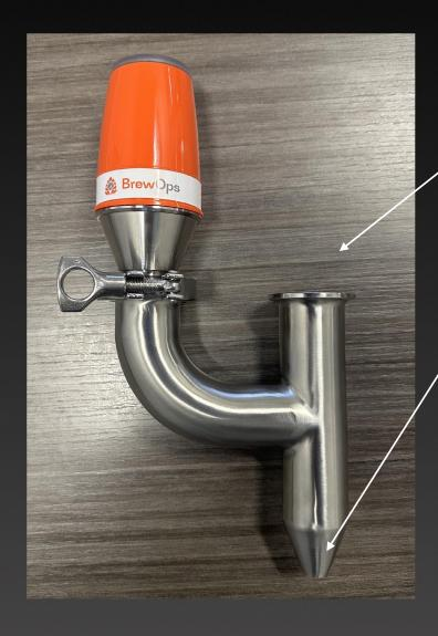
1 1.5" tri clamp connection to brite tank CIP arm
